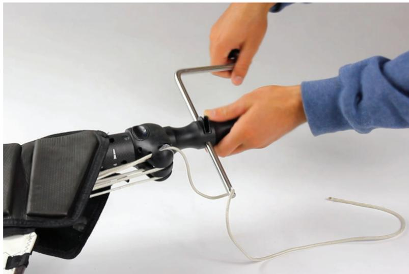
4. Start winching with the line approximately parallel with the mast. As you wind the axel it will automatically shift to the side of the line.
