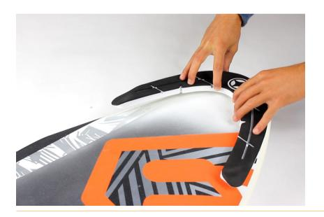
4. After application it is important to continuously apply pressure. At room temperature approximately 50% of ultimate bond strength will be achieved after 20 minutes and 100% after 72 hours. If the Nose Protector comes off due to improper application it is possible to (re)fix the Nose Protector with a Contact Adhesive Gel.
